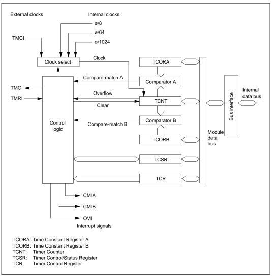
Figure 11-1 Block Diagram of 8-Bit Timer
