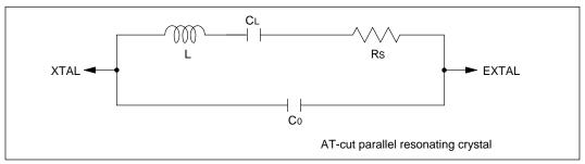
Figure 8-3 Crystal Oscillator Equivalent Circuit
