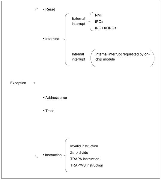
Figure 4-1 Types of Factors Causing Exception Handling
