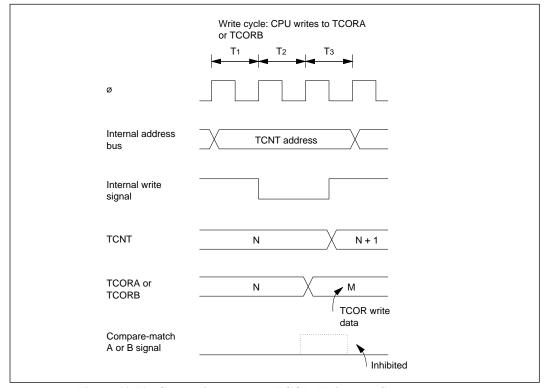
Figure 11-11 Contention between TCOR Write and Compare-Match
