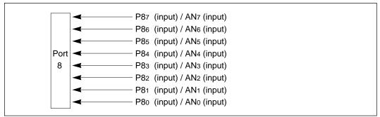
Figure 9-20 Pin Functions of Port 8
