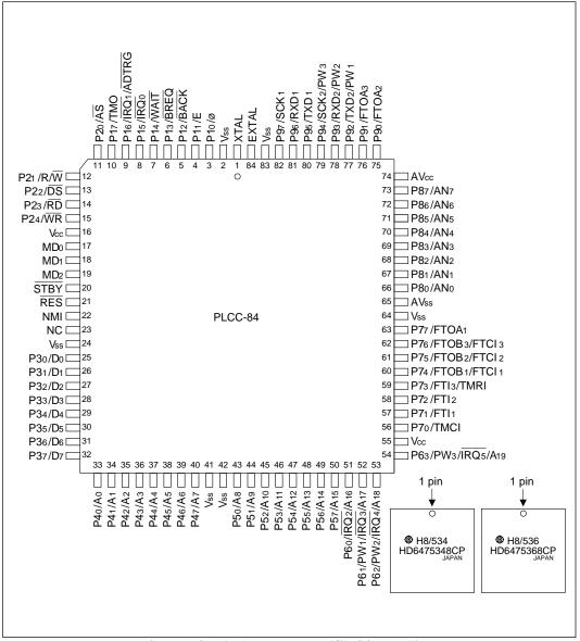
Figure 1-2 Pin Arrangement (CP-84, Top View)
