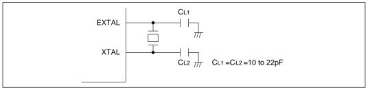
Figure 8-2 Connection of Crystal Oscillator (Example)
