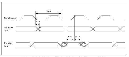
Figure 20-21 SCI Input/Output Timing (Synchronous Mode)
