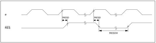
Figure 20-8 Reset Output Timing
