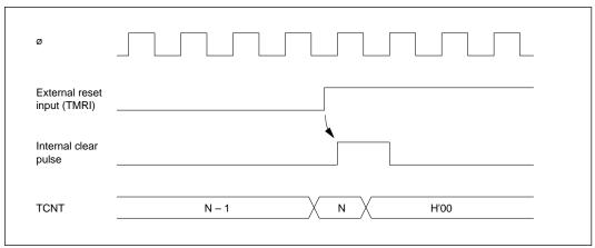
Figure 11-6 Timing of External Reset
