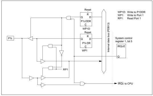
Figure C-1 (f) Schematic Diagram of Port 1, Pin P15
