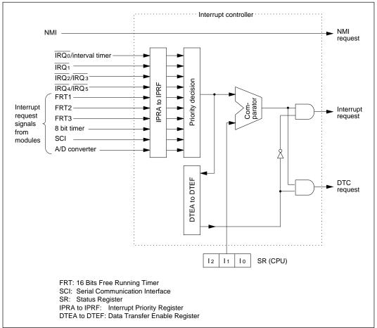
Figure 5-1 Interrupt Controller Block Diagram
