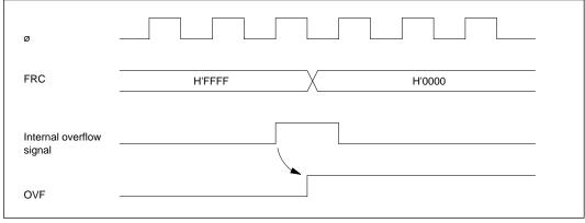
Figure 10-10 Setting of Overflow Flag (OVF)
