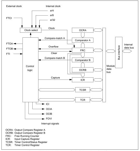
Figure 10-1 Block Diagram of 16-Bit Free-Running Timer
