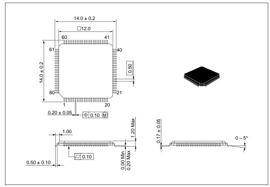
Figure G-4 Package Dimensions (TFP-80C)
