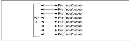
Figure 9-10 Port 4 Pin Functions in Single-Chip Mode
