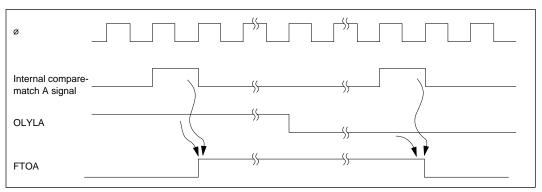
Figure 10-5 Timing of Output Compare A
