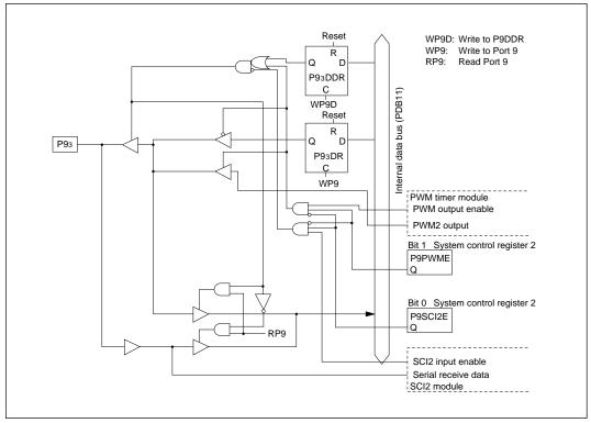
Figure C-9 (c) Schematic Diagram of Port 9, Pin P93
