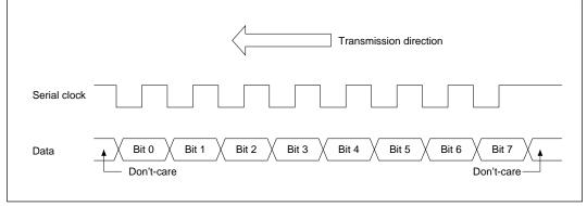
Figure 14-4 Data Format in Synchronous Mode
