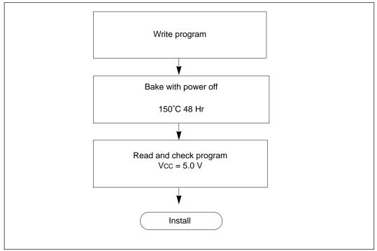
Figure 17-8 Recommended Screening Procedure
