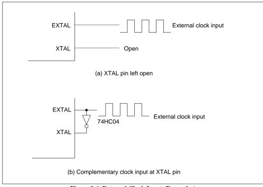
Figure 8-6 External Clock Input (Examples)
