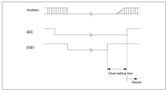
Figure 18-2 Hardware Standby Sequence
