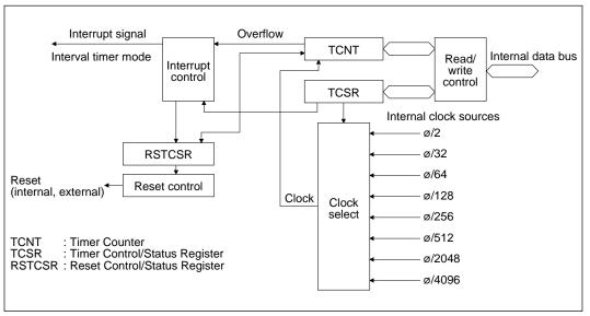
Figure 13-1 Block Diagram of Timer Counter
