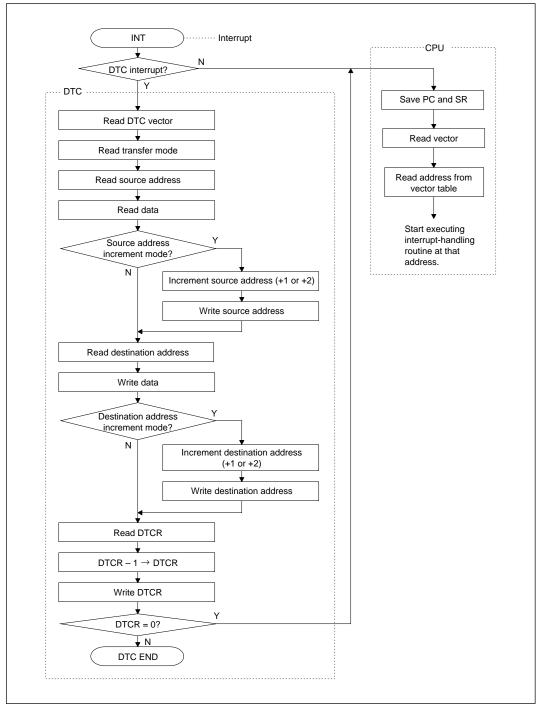
Figure 6-2 Flowchart of Data Transfer Cycle
