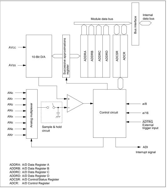
Figure 15-1 Block Diagram of A/D Converter
