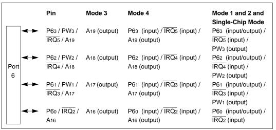
Figure 9-15 Pin Functions of Port 6
