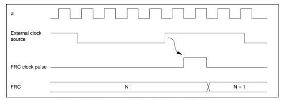
Figure 10-3 Increment Timing for External Clock Input
