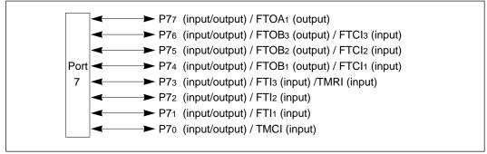
Figure 9-19 Pin Functions of Port 7
