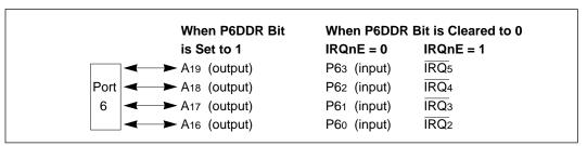
Figure 9-17 Port 6 Pin Functions in Mode 4
