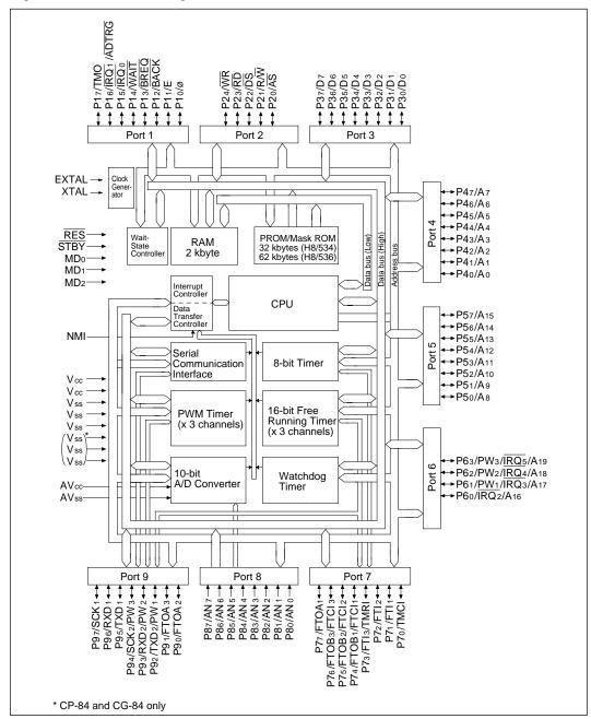
Figure 1-1 Block Diagram
