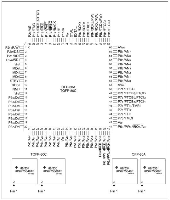
Figure 1-4 Pin Arrangement (FP-80A, TFP-80C, Top View)
