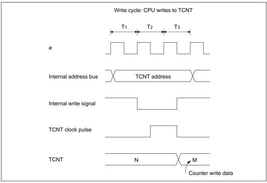
Figure 13-8 TCNT Write-Increment Contention
