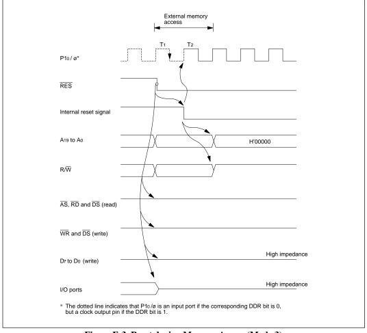
Figure E-3 Reset during Memory Access (Mode 3)
