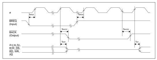
Figure 20-10 Bus Release State Timing
