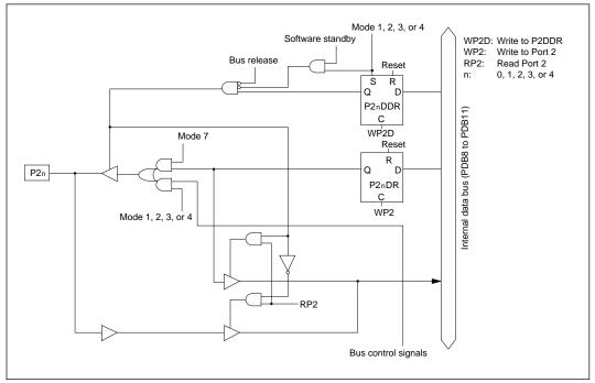
Figure C-2 Schematic Diagram of Port 2
