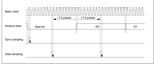
Figure 14-5 Sampling Timing (Asynchronous Mode)
