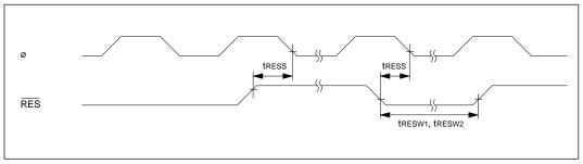
Figure 20-7 Reset Input Timing
