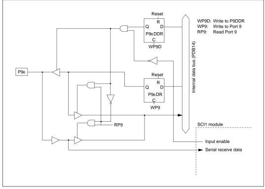
Figure C-9 (f) Schematic Diagram of Port 9, Pin P96
