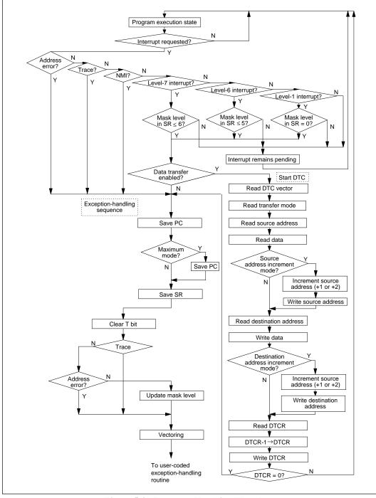
Figure 5-2 Interrupt Handling Flowchart
