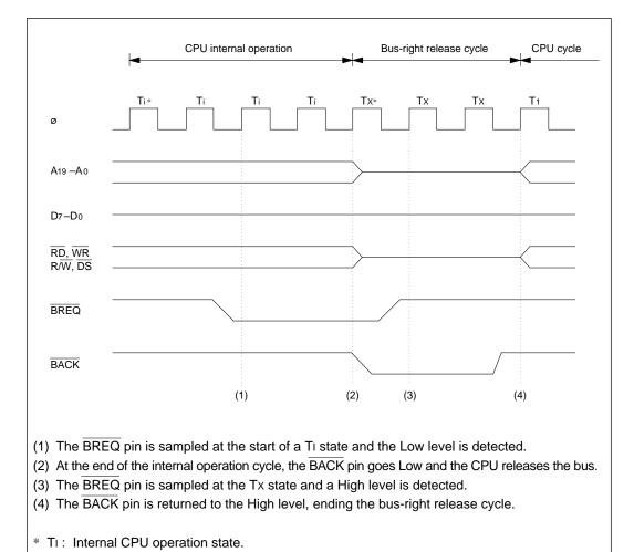
Figure 3-15 Bus-Right Release Cycle (During Internal CPU Operation)
