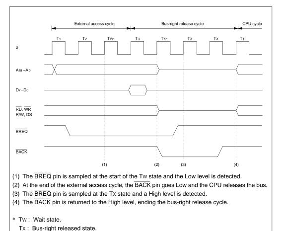
Figure 3-14 Bus-Right Release Cycle (During External Access Cycle)
