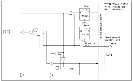
Figure C-1 (c) Schematic Diagram of Port 1, Pin P12
