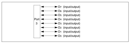
Figure 9-6 Port 3 Pin Functions in Expanded Modes
