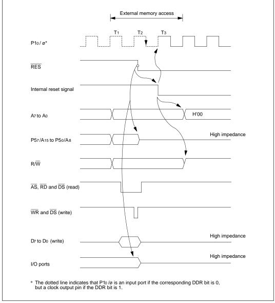
Figure E-2 Reset during Memory Access (Mode 2)
