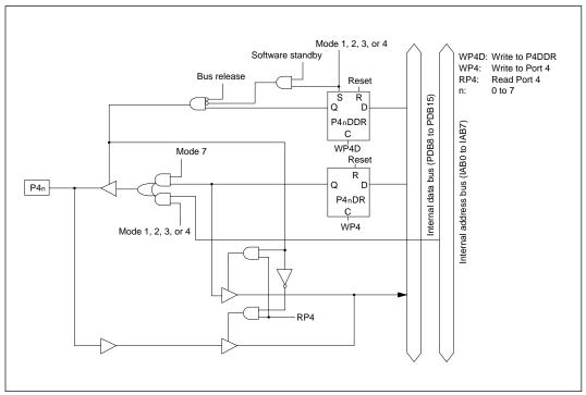
Figure C-4 Schematic Diagram of Port 4
