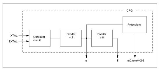
Figure 8-1 Block Diagram of Clock Pulse Generator
