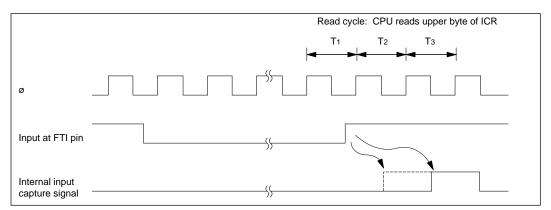
Figure 10-8 Input Capture Timing (1-State Delay)
