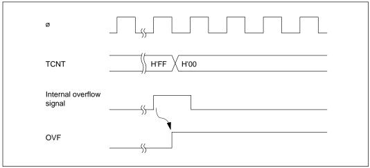
Figure 13-6 Setting of OVF Bit
