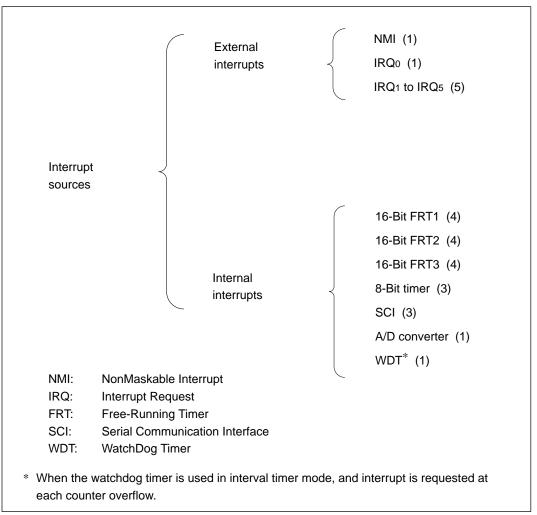
Figure 4-5 Interrupt Sources (and Number of Interrupt Types)
