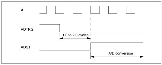
Figure 15-6 Timing of Setting of ADST Bit
