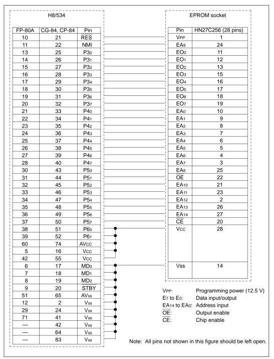
Figure 17-2(a) Socket Adapter Pin Arrangements (H8/534)
