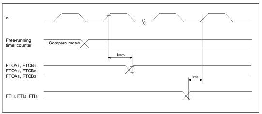
Figure 20-14 Free-Running Timer Input/Output Timing
