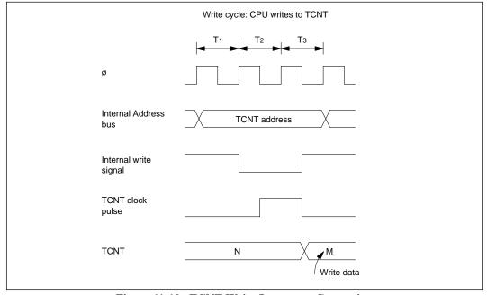
Figure 11-10 TCNT Write-Increment Contention
