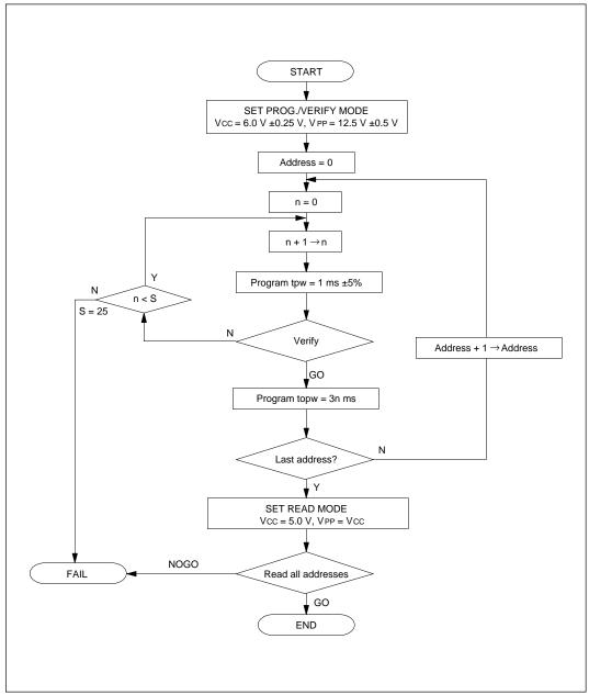
Figure 17-4 High-Speed Programming Flowchart (H8/534)
