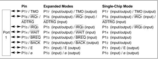
Figure 9-1 Pin Functions of Port 1
