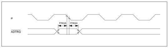
Figure 20-22 A/D Trigger Signal Input Timing
