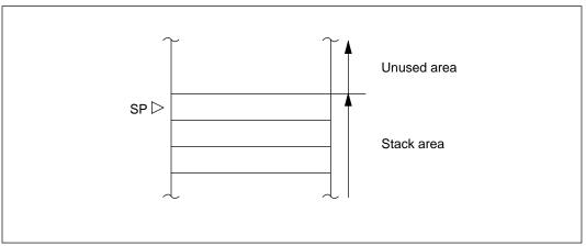
Figure 3-3 Stack Pointer
