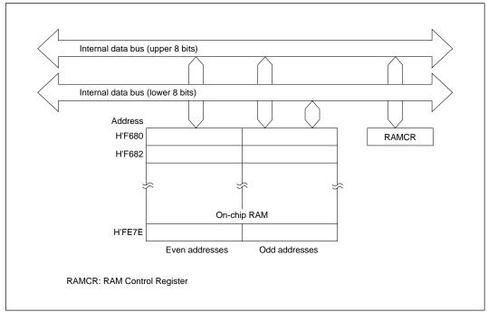
Figure 16-1 Block Diagram of On-Chip RAM
