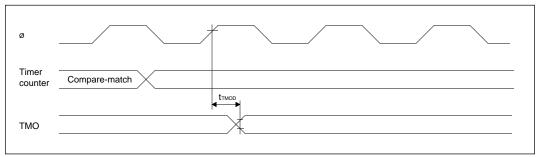
Figure 20-16 8-Bit Timer Output Timing
