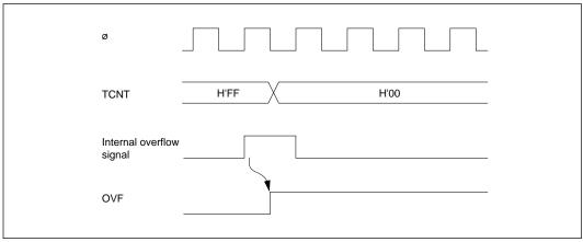
Figure 11-7 Setting of Overflow Flag (OVF)
