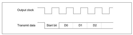
Figure 14-3 Phase Relationship between Clock Output and Transmit Data
