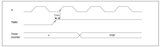
Figure 20-18 8-Bit Timer Reset Input Timing
