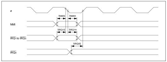
Figure 20-9 Interrupt Input Timing
