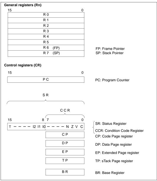
Figure 3-2 Registers in the CPU
