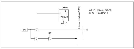
Figure C-1 (b) Schematic Diagram of Port 1, Pin P11
