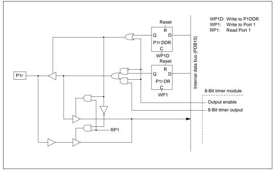
Figure C-1 (h) Schematic Diagram of Port 1, Pin P17
