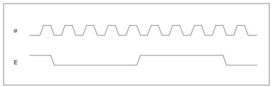
Figure 8-7 Phase Relationship of ø Clock and E Clock
