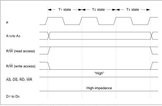
Figure 3-9 Pin States during Register Field Access
