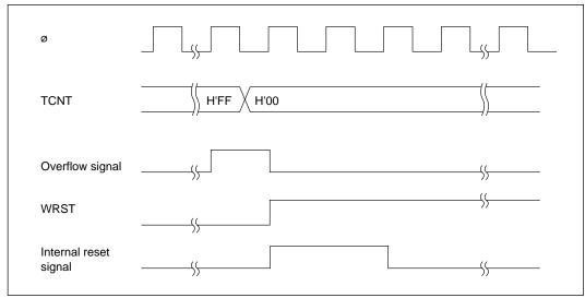
Figure 13-7 Setting of WRST Bit and Internal Reset Signal
