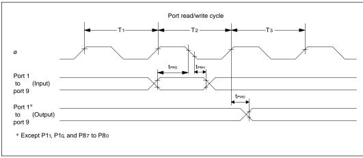
Figure 20-13 I/O Port Input/Output Timing
