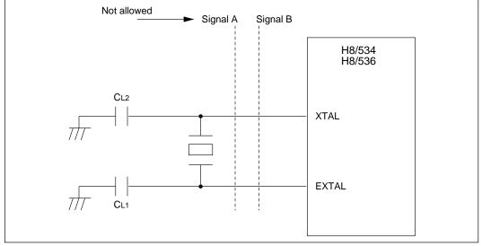
Figure 8-4 Notes on Board Design around External Crystal
