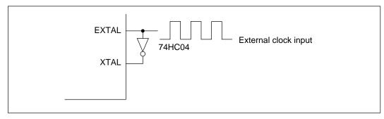
Figure 8-5 External Clock Input (Example)
