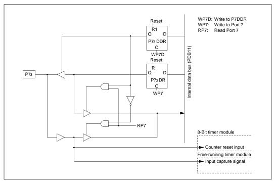
Figure C-7 (c) Schematic Diagram of Port 7, Pin P73
