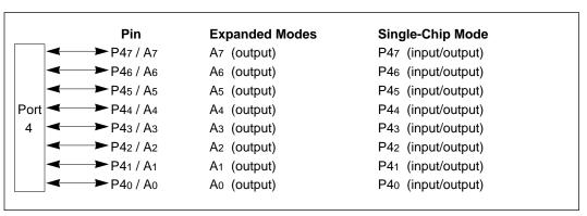
Figure 9-8 Pin Functions of Port 4
