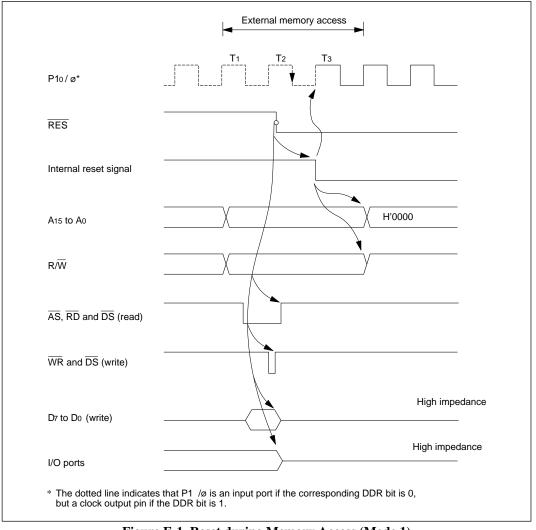
Figure E-1 Reset during Memory Access (Mode 1)
