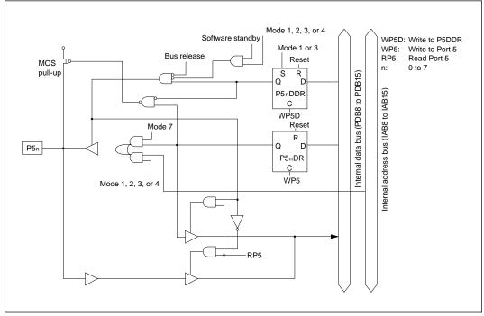
Figure C-5 Schematic Diagram of Port 5
