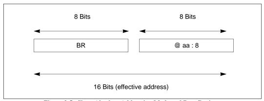
Figure 3-5 Short Absolute Addressing Mode and Base Register
