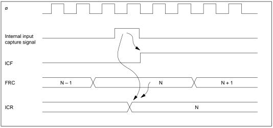
Figure 10-9 Setting of Input Capture Flag
