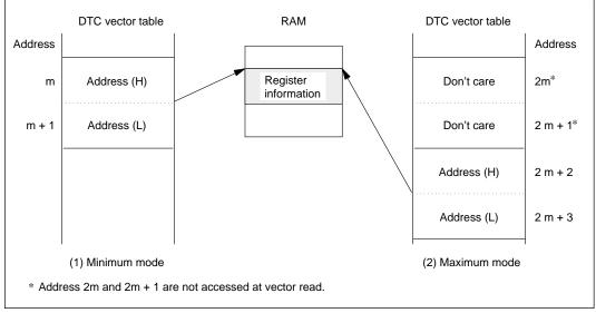
Figure 6-4 DTC Vector Table Entry
