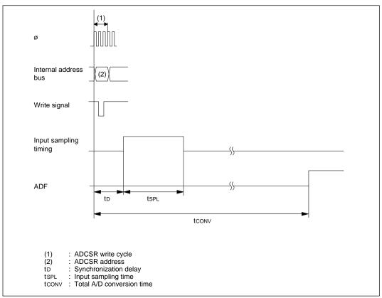
Figure 15-5 A/D Conversion Timing
