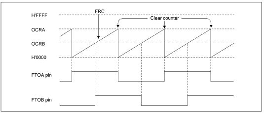
Figure 10-11 Square-Wave Output (Example)
