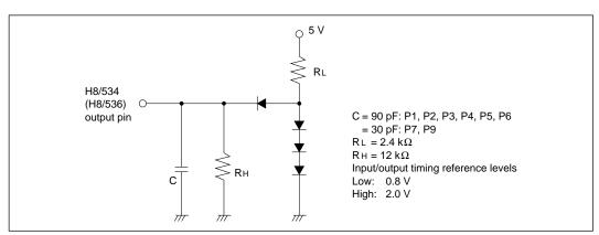
Figure 20-3 Output Load Circuit
