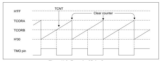
Figure 11-8 Example of Pulse Output
