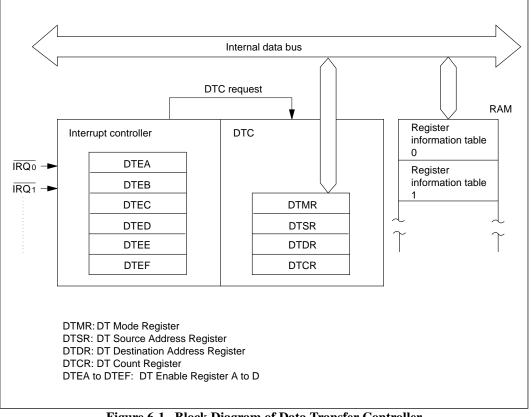
Figure 6-1 Block Diagram of Data Transfer Controller
