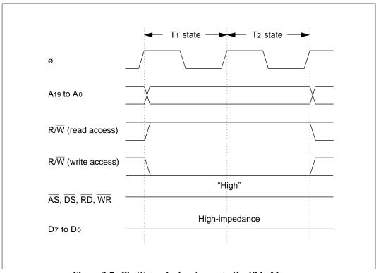
Figure 3-7 Pin States during Access to On-Chip Memory
