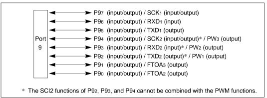
Figure 9-21 Pin Functions of Port 9
