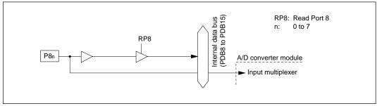
Figure C-8 Schematic Diagram of Port 8
