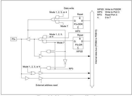
Figure C-3 Schematic Diagram of Port 3
