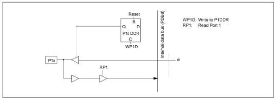
Figure C-1 (a) Schematic Diagram of Port 1, Pin P10
