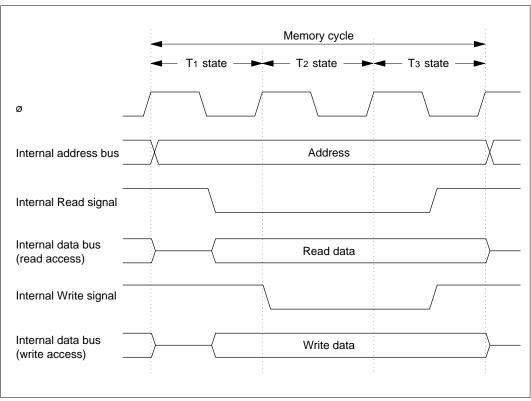
Figure 3-8 Register Field Access Timing
