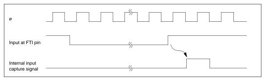
Figure 10-7 Input Capture Timing (Usual Case)
