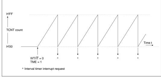
Figure 13-5 Operation in Interval Timer Mode
