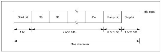
Figure 14-2 Data Format in Asynchronous Mode
