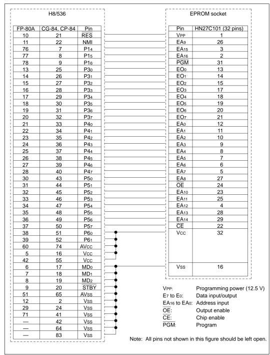
Figure 17-2(b) Socket Adapter Pin Arrangements (H8/536)
