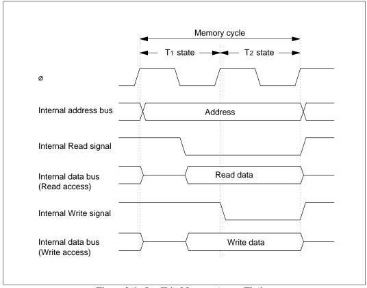
Figure 3-6 On-Chip Memory Access Timing
