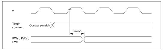
Figure 20-19 PWM Timer Output Timing
