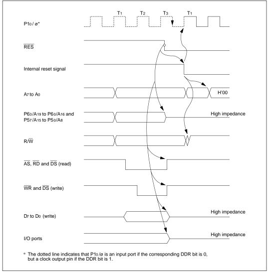
Figure E-4 Reset during Memory Access (Mode 4)
