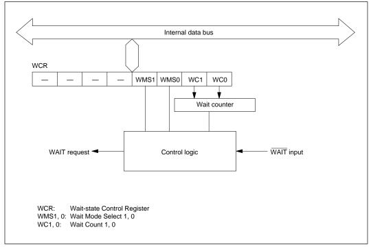
Figure 7-1 Block Diagram of Wait-State Controller
