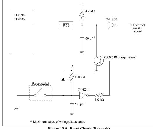
Figure 13-9 Reset Circuit (Example)
