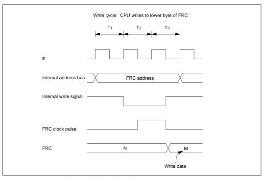
Figure 10-13 FRC Write-Increment Contention
