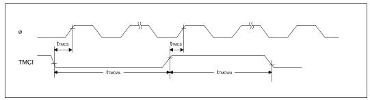
Figure 20-17 8-Bit Timer Clock Input Timing
