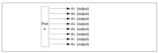
Figure 9-9 Port 4 Pin Functions in Expanded Modes
