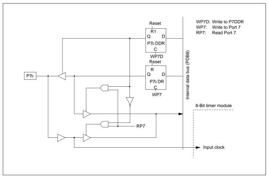
Figure C-7 (a) Schematic Diagram of Port 7, Pin P70
