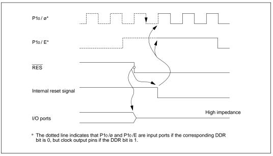
Figure E-5 Reset during Memory Access (Mode 7)
