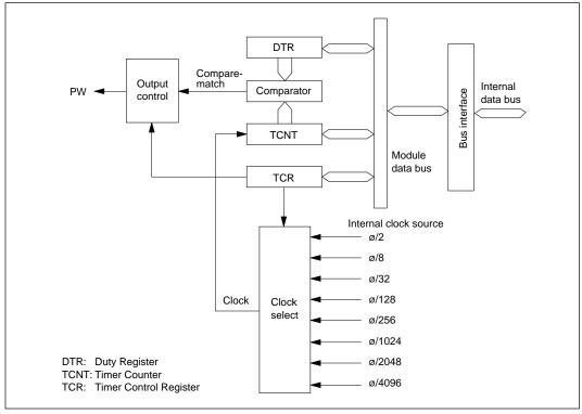
Figure 12-1 Block Diagram of PWM Timer
