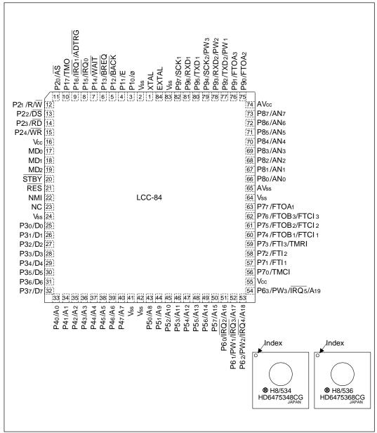
Figure 1-3 Pin Arrangement (CG-84, Top View)
