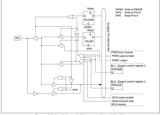
Figure C-9 (b) Schematic Diagram of Port 9, Pin P92
