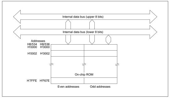
Figure 17-1 Block Diagram of On-Chip ROM
