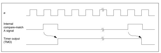
Figure 11-4 Timing of Timer Output
