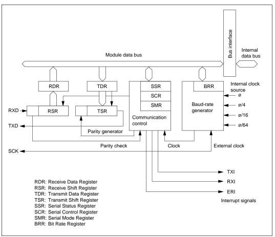
Figure 14-1 Block Diagram of Serial Communication Interface
