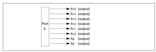
Figure 9-12 Port 5 Pin Functions in Modes 1 and 3
